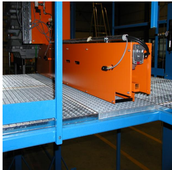
Low maintenance accurate and simple pneumatic linear cylinder for strapping bayonet drive
